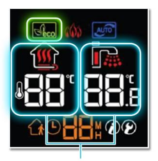
The display on the left shows Heating The display on the right shows the domestic hot water
