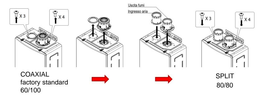
COAXIAL FUMISTERY: maximum equivalent length allowed **30m** \*Curve 90 = -2m / Curve 45 = -1m / max 3 curves 90 or 6 curves 45
